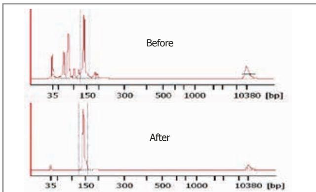
Using a PippinHT, unwanted artifacts can be removed from microRNA libraries using a range setting. 24 samples can be processed with a 30 minute run time.
