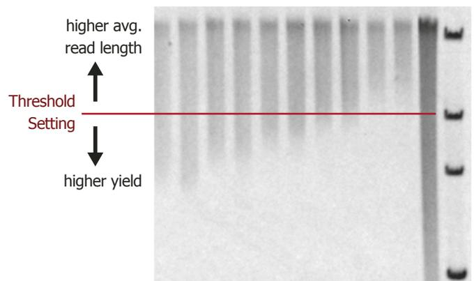
High-pass removal of smaller DNA lets 3rd-gen sequencers focus on the longest fragments.
